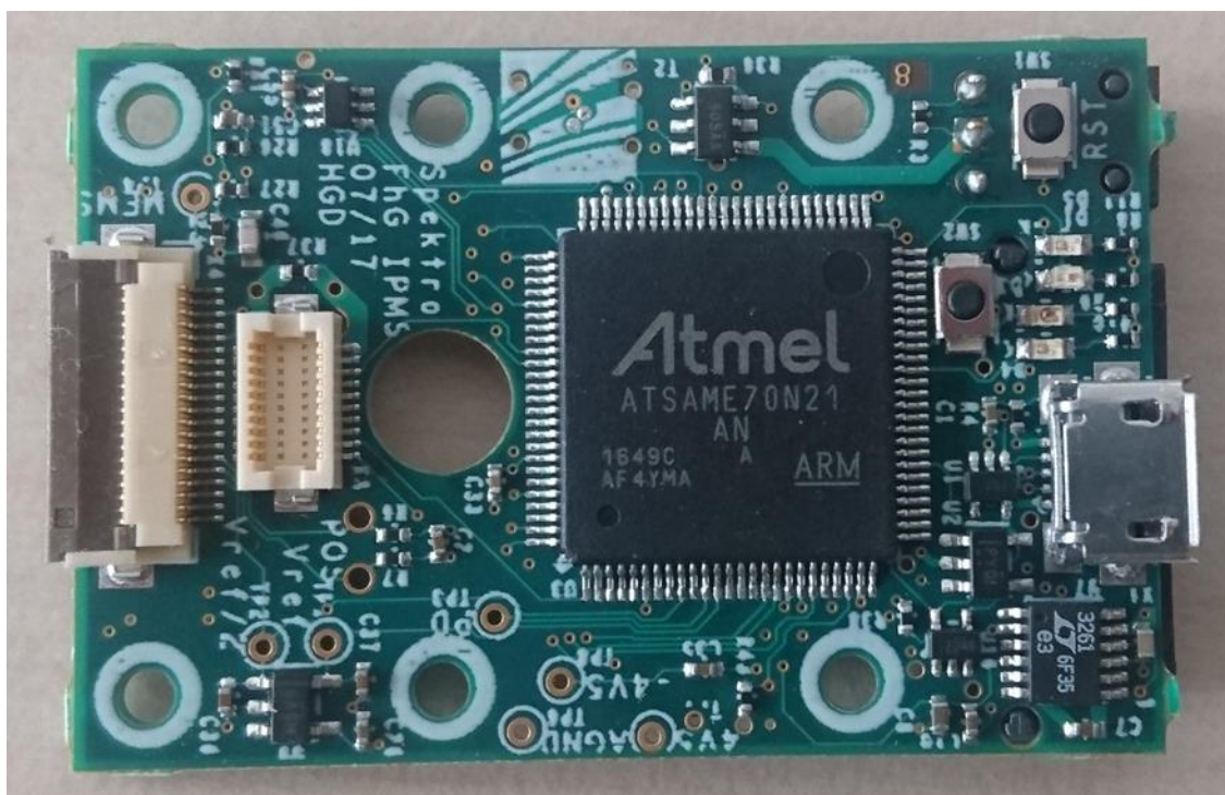
Figure 9 - Super-ordinated PhasmaFOOD driving board for the IPMS NIR spectrometer module.
